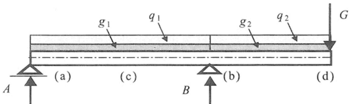
Figure 3: Beam with overhangs - a decisive combination for determining the maximum reaction B and extreme bending momentum at point b (EQU, STR).  $\gamma_{g1} = 1,35$ ,  $\gamma_{g2} = 1,35$ ,  $\gamma_G = 1,35$ ,  $\gamma_{q1} = 1,5$ ,  $\gamma_{q2} = 1,5$
