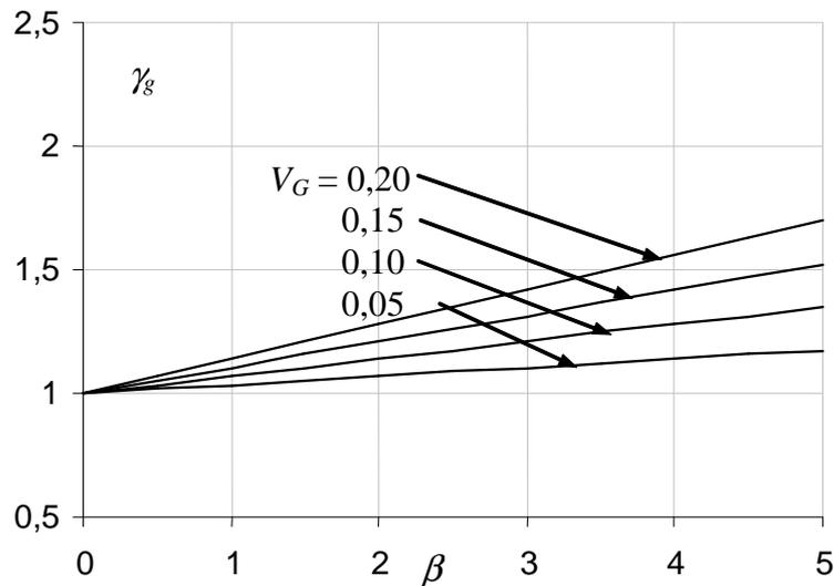
Fig. B.5. Variation of the partial factor  $\gamma_G$  with the reliability index  $\beta$  for selected values of the coefficient of variation  $V_G$
