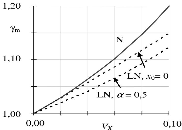
Fig. B.4. Variation of  $\gamma_m$  with  $\beta$  for selected coefficients of variation  $V_X$ , normal and log-normal distribution of  $X$
