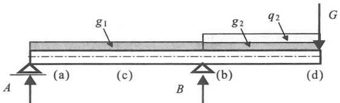
Figure 4: Beam with overhangs - a decisive combination for determining the static balance (reaction A) (EQU).  $\gamma_{g1} = 0,9$ ,  $\gamma_{g2} = 1,1$ ,  $\gamma_G = 1,1$ ,  $\gamma_{q1} = 0,0$ ,  $\gamma_{q2} = 1,5$
