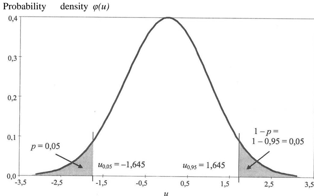
Figure 1: The upper and lower quantile of standardized random quantity  $U$  (in this case  $G$ ) with normal distribution.
