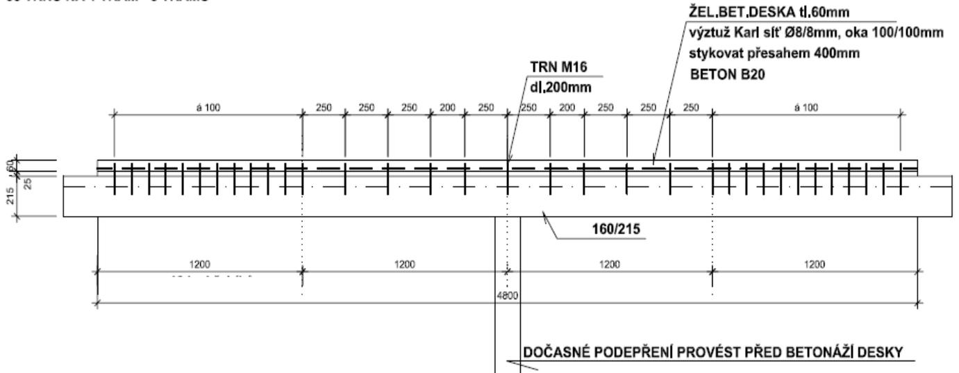
Figure 7 – beam- slab interconnection
