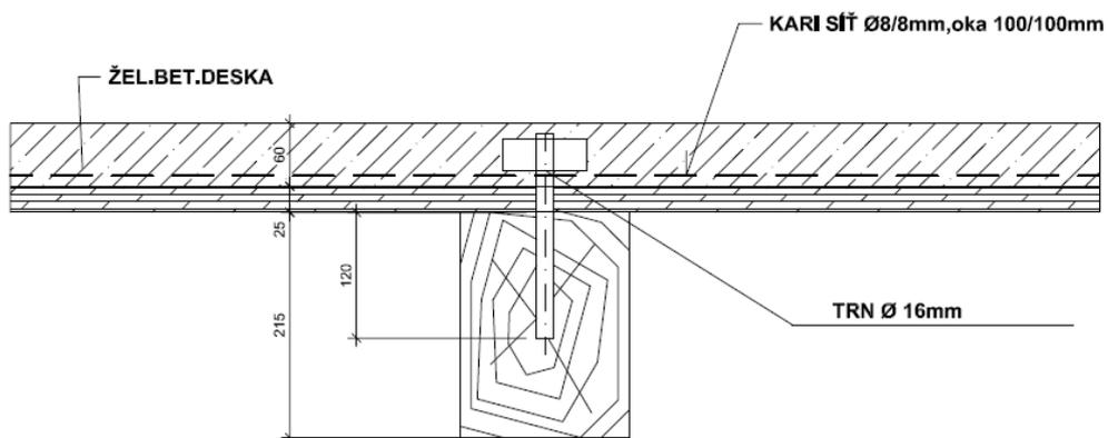
Figure 8 – beam- slab interconnection - section
