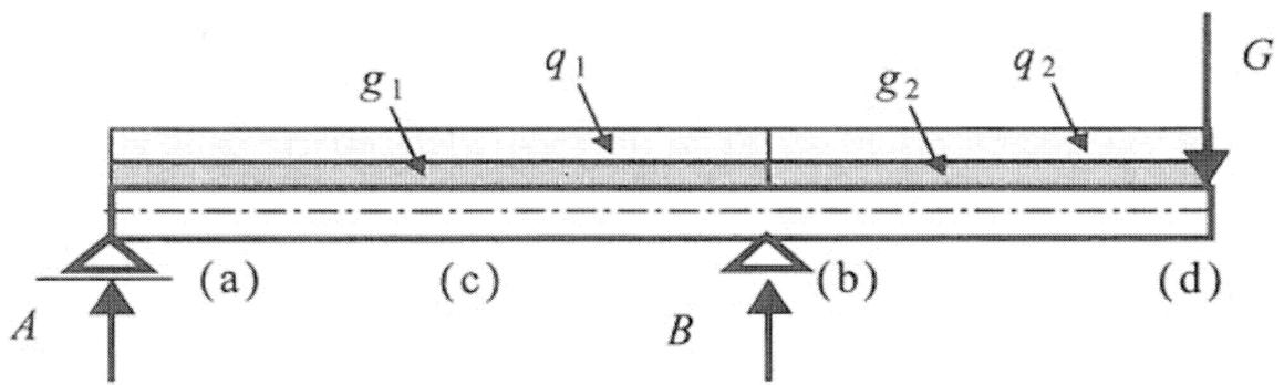
Figure 2: Beam with overhangs - assuming three independent permanent loads  $g_1, g_2, G$  and two independent variables loads  $q_1, q_2$ .
